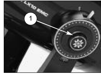
Fig.10: (1) Declination (Dec) Lock.
