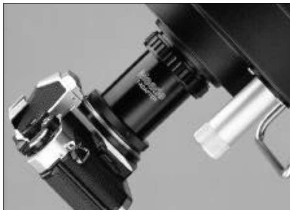
Fig.20: 35mm camera mounted to telescope with T-Adapter.
