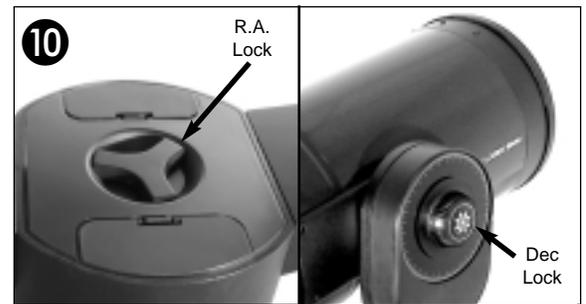
10. Tighten, to a firm feel only, the Dec and R.A. locks (6 and 9, Fig. 1). See page 7 for more information. Remove the dust cover from the end of the telescope tube.
