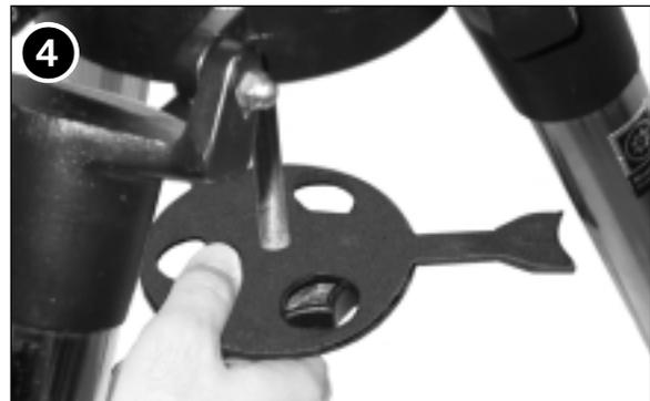
4. Remove the spreader bar (see above figure) from the shipping carton. Slide the spreader bar onto the threaded rod and position the rod back through the tripod head. Place the "C" clip into the slot in the threaded rod – this clip holds the threaded rod in place. Position the spreader bar so that its three arms line up with the three tripod legs.
