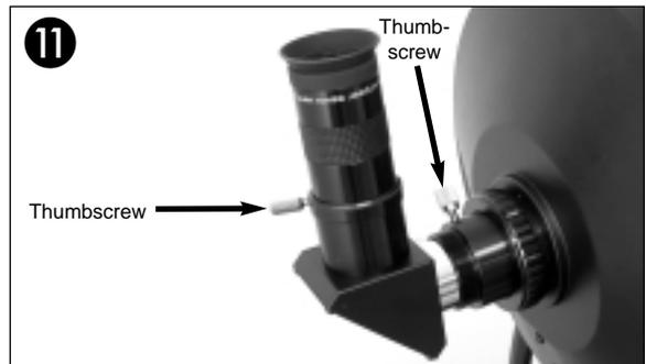
11. Remove the dust cap from the rear cell of the telescope. Thread the eyepiece holder into the rear cell thread. Slide the diagonal prism into the eyepiece holder and lock in place by turning the thumbscrew to a firm feel.
