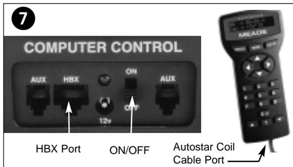
7. Slide the computer control panel power switch to OFF, if necessary. Remove the Autostar handbox and the Autostar interface cable from the packing materials. Plug one end into the HBX port of the computer control panel and plug the other end into the Coil Cable port on the Autostar handbox.
