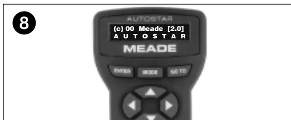
8. Flip the Power Switch on the computer control panel to the ON position. The copyright message lights on Autostar's LCD display.
