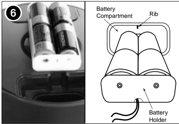
6. Remove the covers from both battery compartments located on top of the drive base and carefully lift the battery holders from their compartments, being mindful of the connector wires. Insert four (user-supplied) C-cell batteries into each battery holder (eight batteries total), oriented as shown on the diagram on the battery holder.
