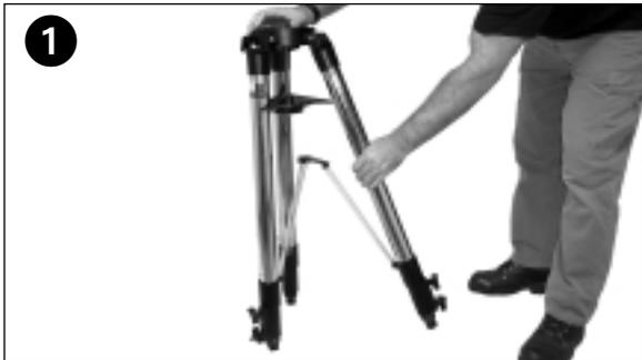
1. Remove the field tripod from the shipping carton. Stand the tripod vertically with the tripod feet down and with the tripod still fully collapsed. Grasp two of the tripod legs and, with the full weight of the tripod on the third leg, gently pull the legs apart to a fully open position.
