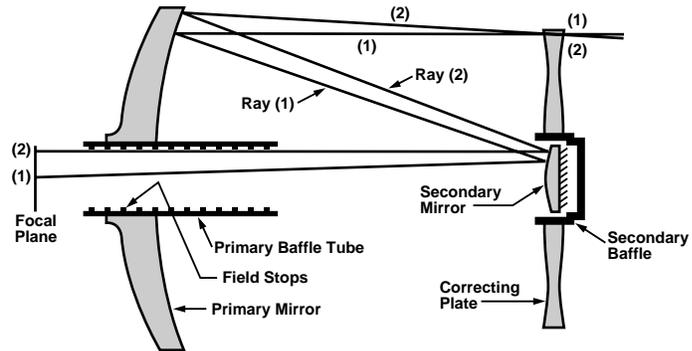
In the Schmidt-Cassegrain design of the Meade LX90, light enters from the right, passes through a thin lens with 2-sided aspheric correction ("correcting plate"), proceeds to a spherical primary mirror, and then to a convex secondary mirror. The convex secondary mirror multiplies the effective focal length of the primary mirror and results in a focus at the focal plane, with light passing through a central perforation in the primary mirror.
